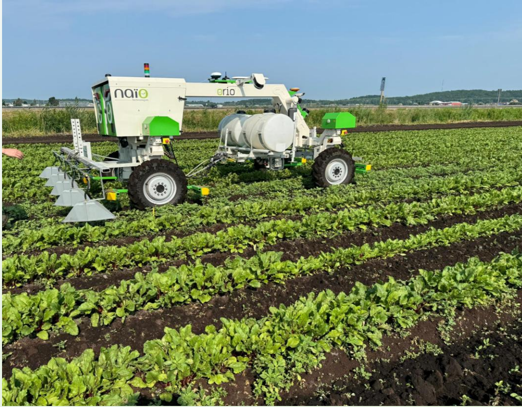
Naïo Orio with band sprayer and two 55-gallon tanks
