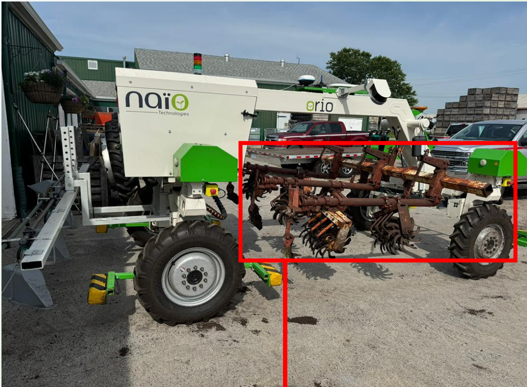
Naïo Orio fitted with the rolling gang cultivator with spider spikes
