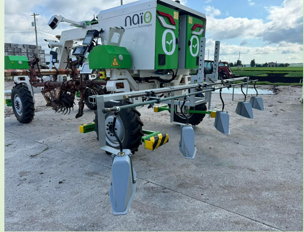
Naïo Orio with band sprayer and two 55-gallon tanks
